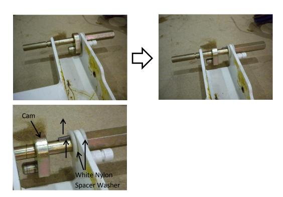
4) Slide the old hex shaft out of the lower carriage
