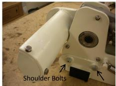
2) Carefully lift the top half from the lower carriage then slide sideways to remove the cam from the push rod. Then remove the return spring.
