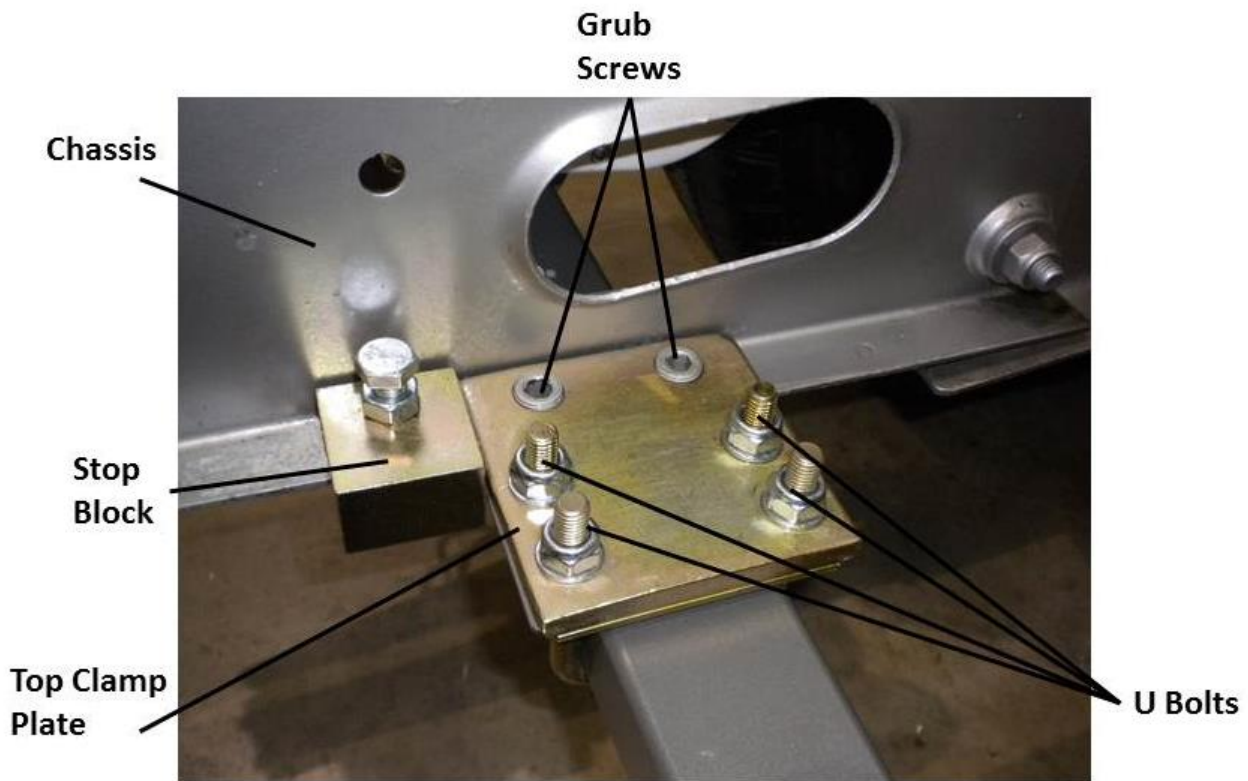
FIG 2: CLAMP ASSEMBLY WITH STOP BLOCK
