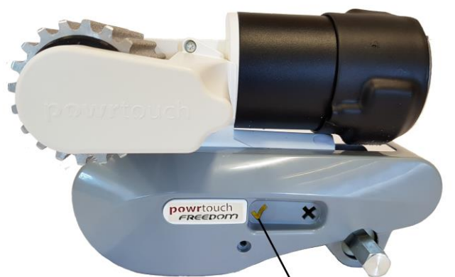
Roller Position Indicator Showing roller in the ON position
