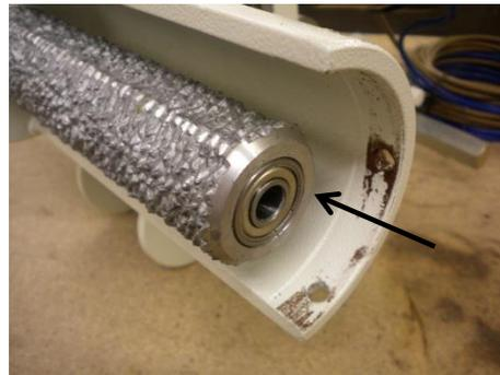
8) Replace roller end cap and re-tighten the 3 x M6 screws (10mm hexagon head) to 7.5nm
